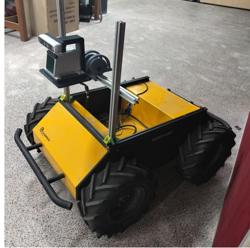
Figure 4. Hardware setup: Sensor mounting on Husky UGV.
